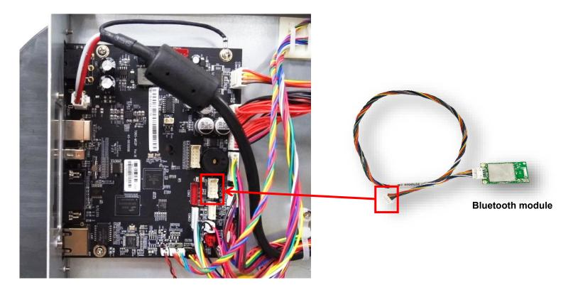
5. Reassemble the parts in the reverse procedures.
