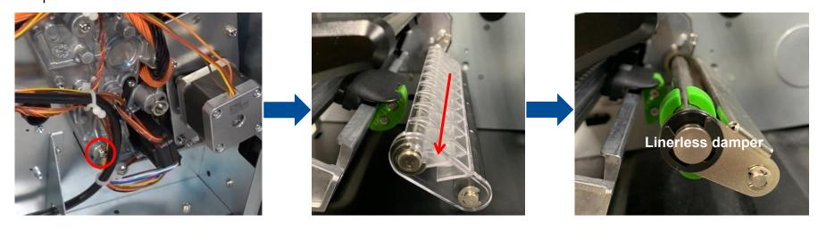
10. Plug the tear (or cutter) module mini DIN cable connector into the printer receptacle.
