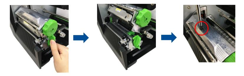
5. Disconnect the printhead harness to remove/replace the new printhead assembly.
