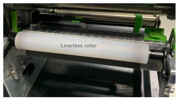
7. Remove the two screws and replace the cover (green) from plastic to rubber.
