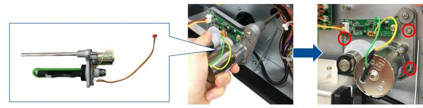
5. Connect the rewinder module cable to the main board socket (CON26/ red).
