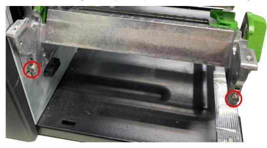
5. Move the label guide (green) to the outermost side to install the rubber cover and stick the linerless pad on the lower base.
