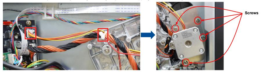
4. Remove/Replace the stepping motor assembly. (including gears and stepping motor)
