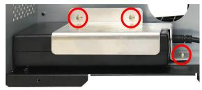
4. Remove one screw (fastened by 7.5 kg±15% kg-cm) and disconnect one connector on main board. Loosen three cable ties to remove/replace the power supply unit.
