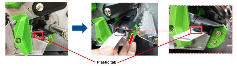
5. Remove/Replace the gap/black mark sensor.
