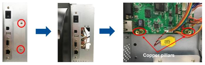
Note: Refer to Slot-in Wireless Housing Installation (Option) to remove the housing. (if module installed)
