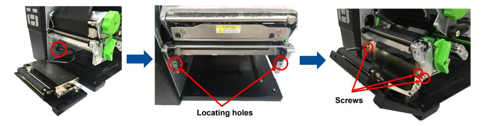
4. Close the peel-off sensor module and complete installation.
