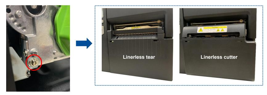
12. For the linerless cutter module, the cutter tray is mounted on the cutter panel as required.
