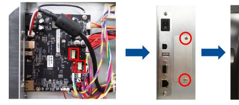
4. Install the slot-in wireless housing on the rear of the printer and fix the two screws. (5.5 kg±15% kg-cm) Connect another side of the cables to the slot-in wireless transfer module housing board. Reassemble the parts in the reverse procedures.
