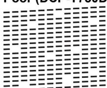
6. When the LCD message prompts you to check the print quality of each colour, press **▲** or **▼** to select the pattern that most closely matches the printing result. Press **OK**.
